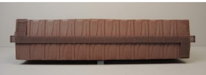
Photo 10: Apex running board installed.
