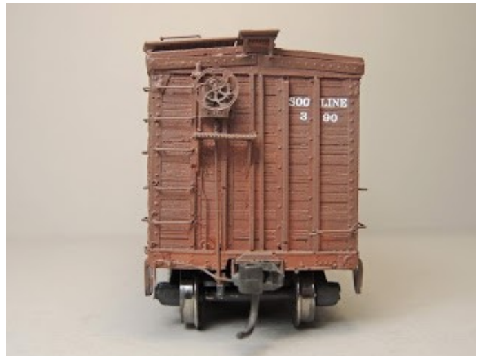
Photo 3: Note added posts in center of end above coupler, triangular shape and rivet strip above posts.
