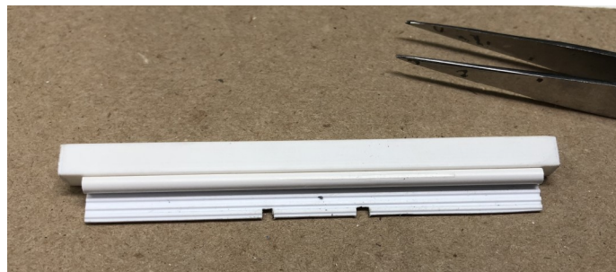
Photo 1: The completed upper door assembly. The notches are in the door, and gauged to the track. They go over the rails to fully seal the bottom.
