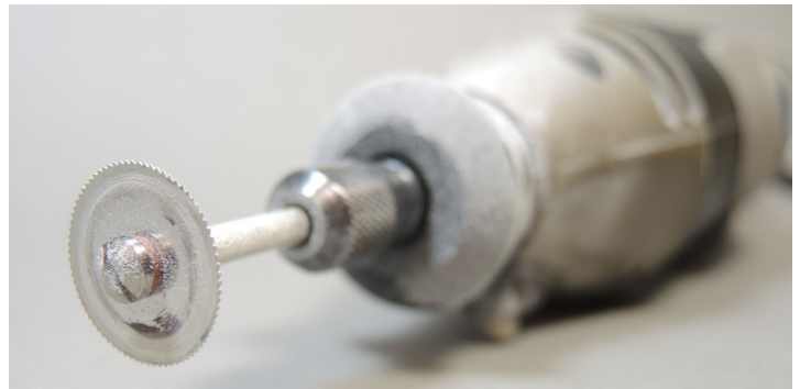
Photo 6: This rotary blade is a mini circular saw, and requires a steady hand and extra care to avoid injury.
