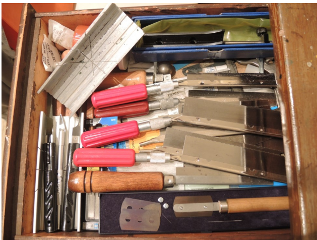
Photo 1: Les' drawer of saws. Note the different blade shapes, widths and miter box.
