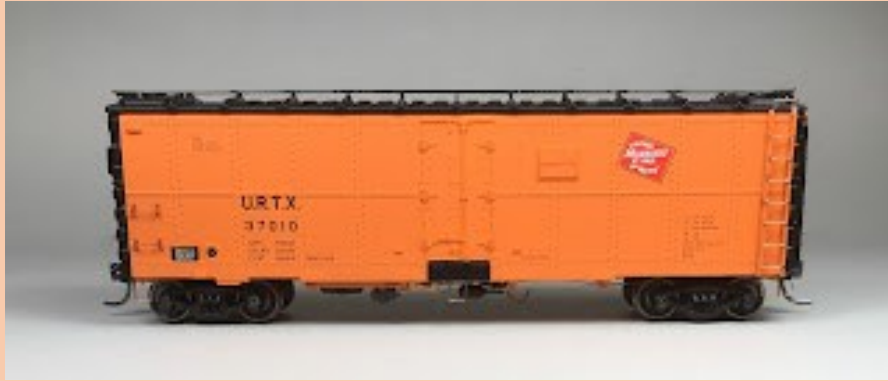
Bracket grab irons and sill steps installed.
