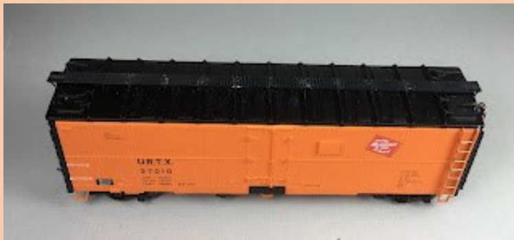
Ladder rungs replaced with wire rungs.
