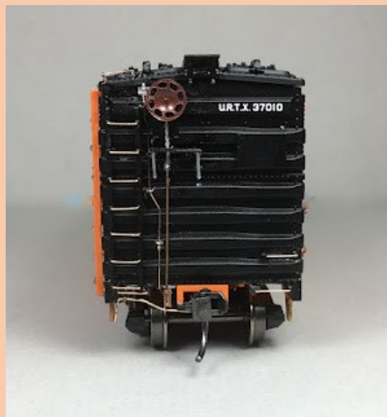
B end with details installed.
