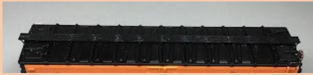
Roof with running board and grab irons installed.
