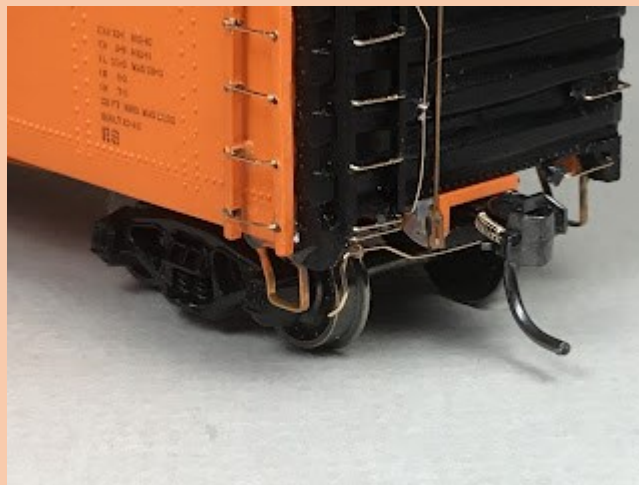
Uncoupling lever angle view. Also note metal sill step installed.
