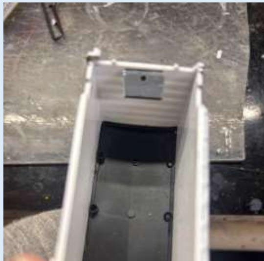
Modeler's Tip - This is how I attach floors after having weights come loose
