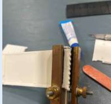
Step 3 - Clamp in action. Apply ACC from the inside
