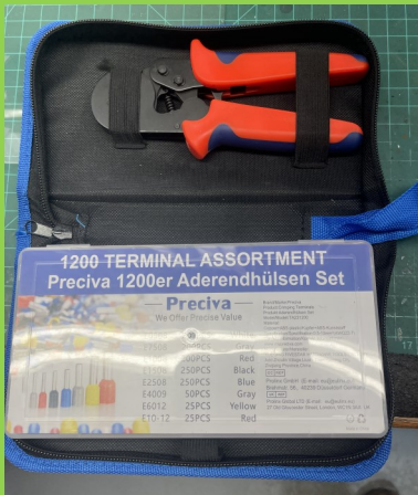
Terminal Crimping Tool Kit with supply of terminal ends for various gauges of wire. Mine came in a nice case
