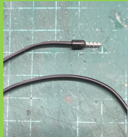
Wire with terminal end crimped on
