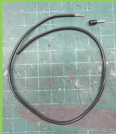
Wire before crimping terminal end
